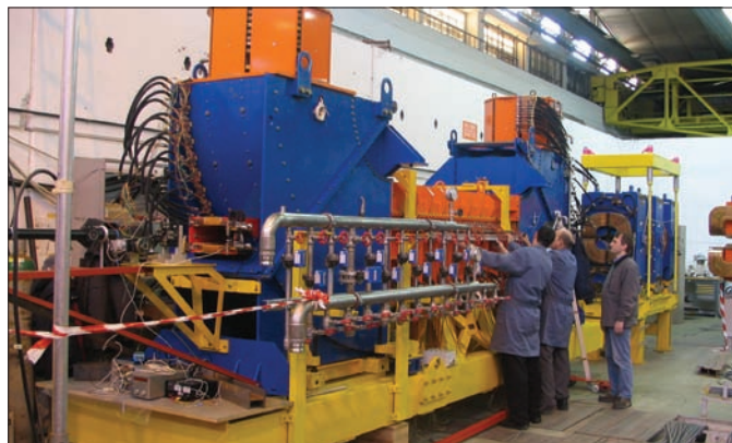
The new cooler for the LEIR ring to provide ion beams for the LHC.
